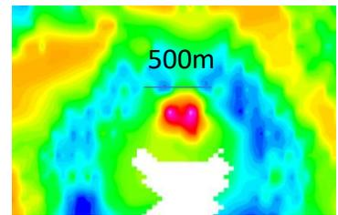
**Middle images:** Model of 600m x 220m conductive plate which may be caused by VMS mineralisation. See Figure 4 for explanation of profiles.
