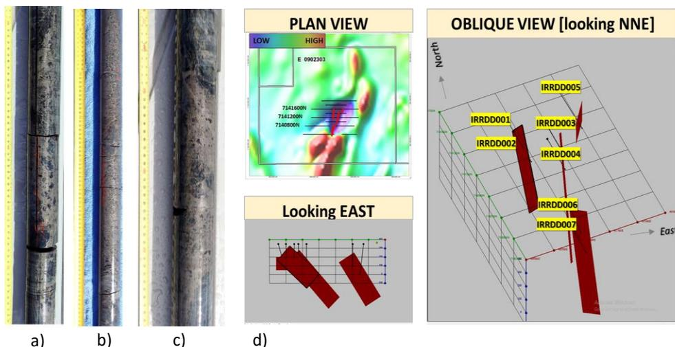
**Figure 1: Irrida Hill drilling** a) Sulphide core from 162m IRRDD002 b) IRRDD004, 222m c) IRRDD002, 163m d) Section, plan and oblique view of Irrida Hill EM plate modelling
