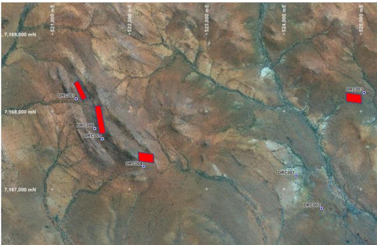
Figure 7. Dingo Pass Drill Hole Location Plan. Red squares - location of untested conductors modelled from DHEM
